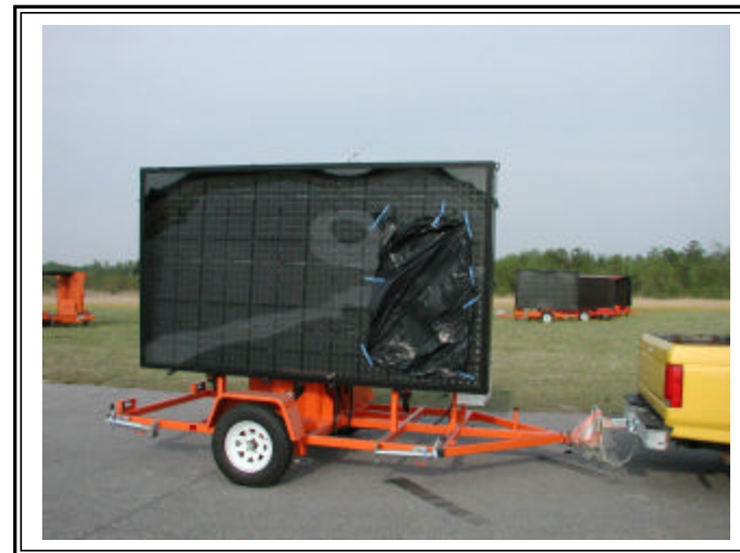
Photocell covering for dimming measurement
